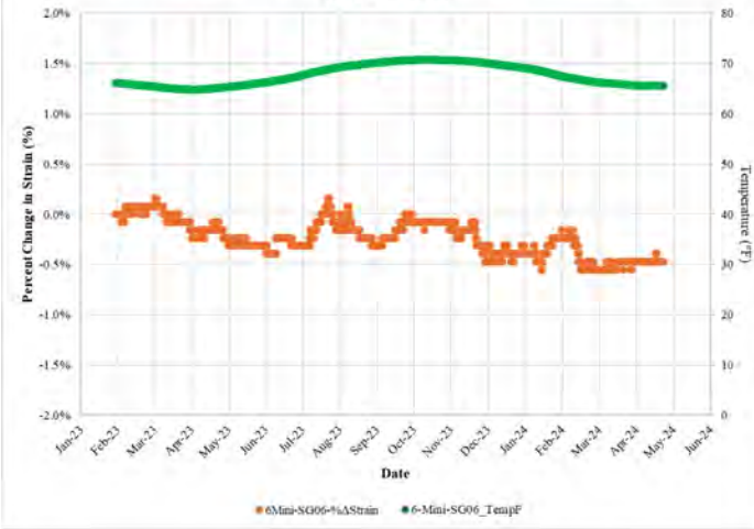
CAISSON #6: Percent Change in Strain and Temperature vs. Time (Depth = 30 ft)
