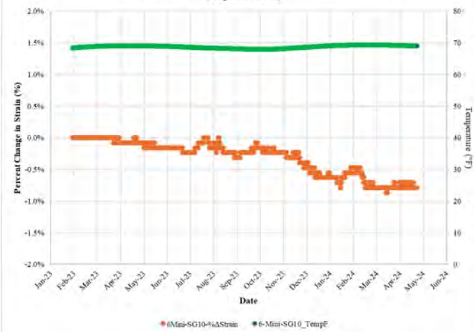
CAISSON #6: Percent Change in Strain and Temperature vs. Time (Depth = 70 ft)
