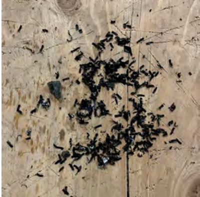
Purging & flushing to remove air and debris in loops
