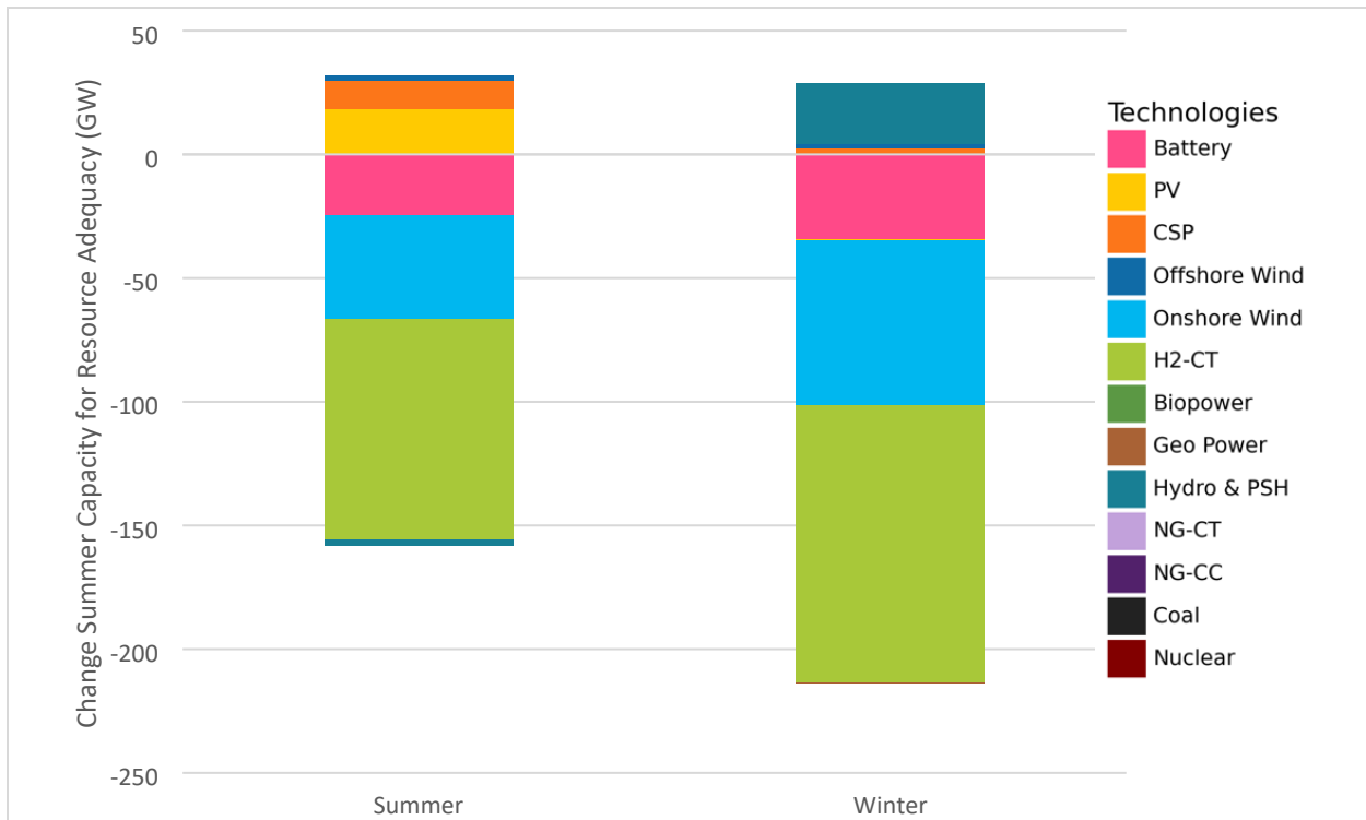
Figure 4-12. Change in summer and winter RA eligible capacity contribution by technologies in the EFS scenario resulting from the mass GHP deployment (including weatherization in SFHs) instead of the partial electrification using ASHPs.
