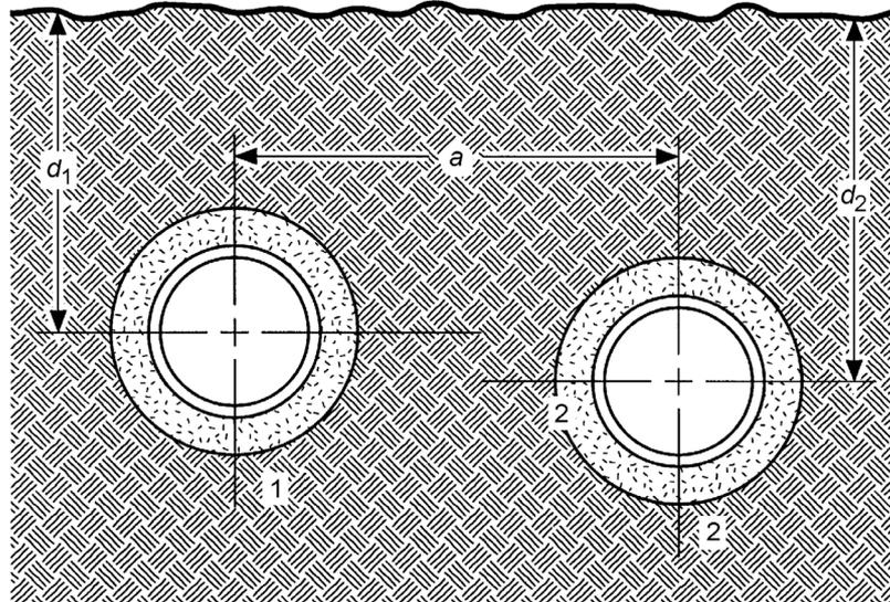
Nomenclature for two buried pipes, Fig. 4.11, DCG;
